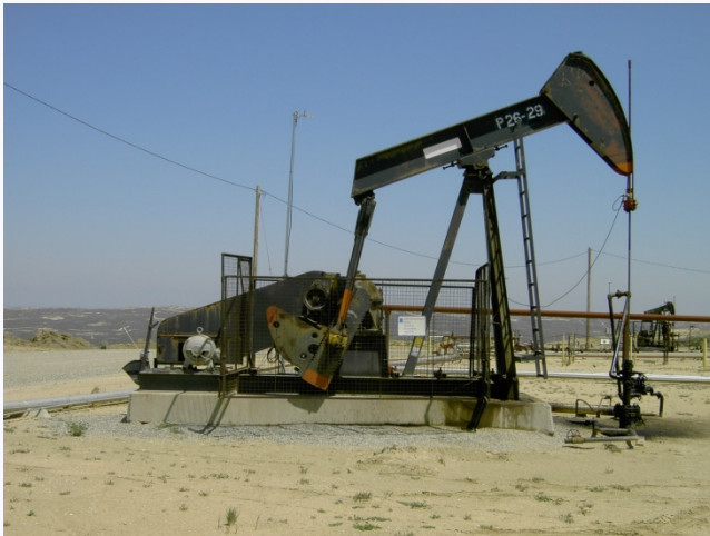
Traditional Surface Pumping Unit (Sandstones and Non-Thermal Diatomite)
